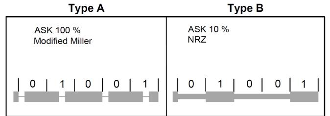
Fig. 3: Reader to card modulation and bit coding definition (taken from [3])
