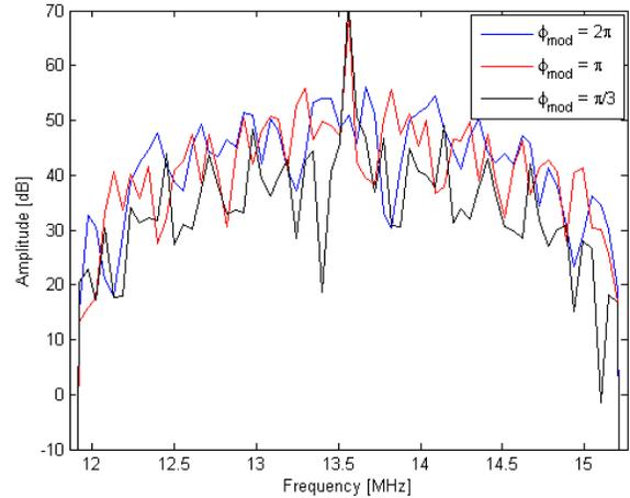
Fig. 8: Spectrum of the 16-PSK at different phase modulation angles at 6.78 Mbit/s
