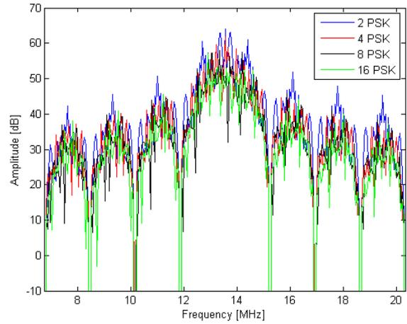
Fig. 7: Spectrum of different PSK orders at data rates up to 6.78 Mbit/s
