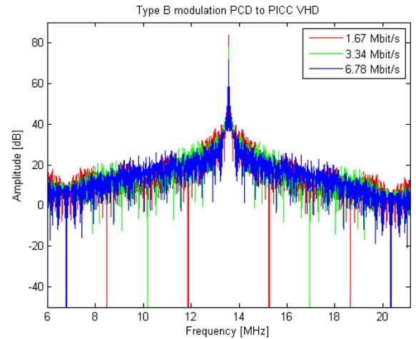
Fig. 5: Frequency spectrum of Type B method at VHDR
