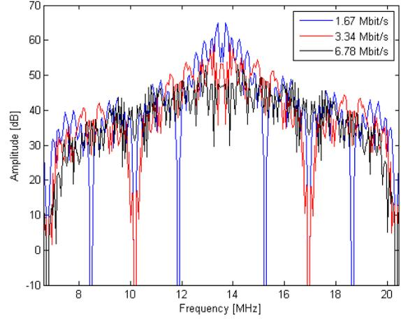
Fig. 6: Spectrum of 2PSK at different data rates up to 6.78 Mbit/s
