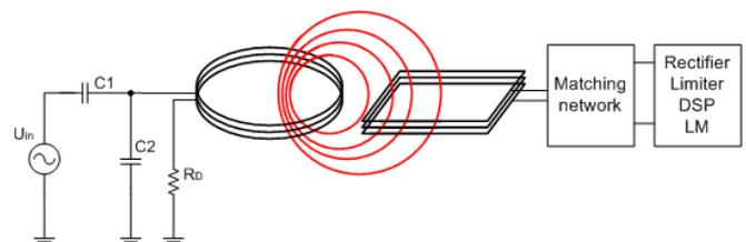
Fig. 1: Principle schematic of an RFID communication system
