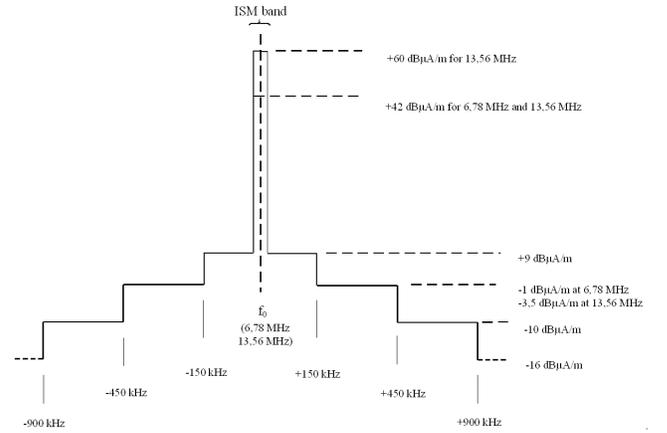
Fig. 2: Spectral mask for 13.56 MHz RFID systems (taken from [8])
