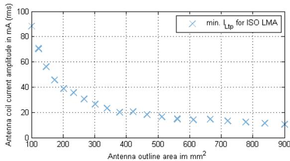
Fig. 12. Minimum required current per conductor turn as function of loop antenna size, to achieve ISO/IEC SBA standard compliance [12].
