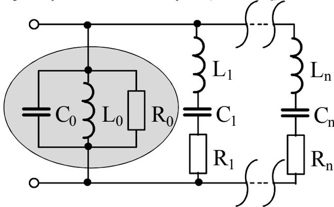
Fig. 2. Ladder network representing the equivalent network of the antenna.
