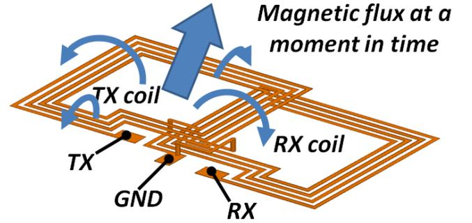
Fig. 5. Layout of the symmetric zero-coupling loop antenna conductor.
