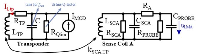
Fig. 11. Equivalent network for NFC device and measurement set-up.
