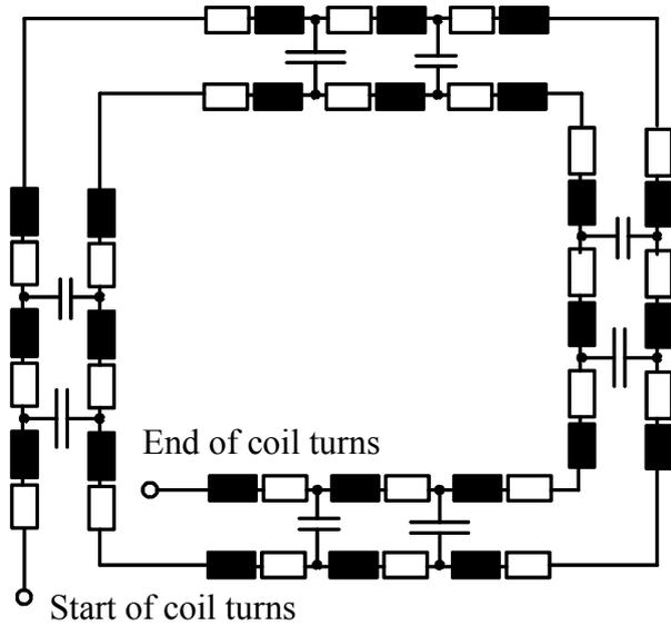
Fig. 1. Loop antenna as distributed component (similar to [10]).
