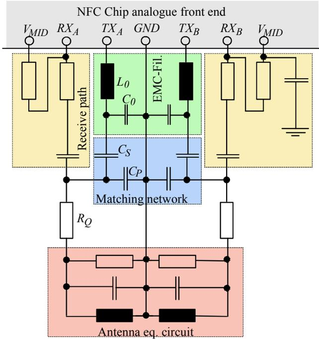
Fig. 9. Differential matching network and EMC filter topology.
