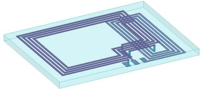
Fig. 13. Asymmetric ALM antenna, optimized for smallest area in NFC card mode.
