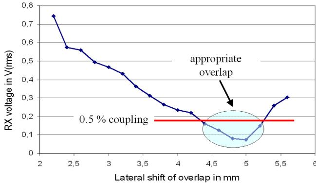
Fig. 6. Optimizing loop overlap for minimum coupling in HFSS simulation.
