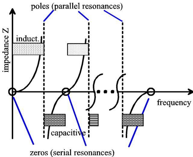
Fig. 3. Impedance of the loop antenna over a wide frequency range.
