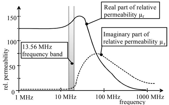
Fig. 4. Relative permeability of ferrite foils for alternating  $H$ -field.
