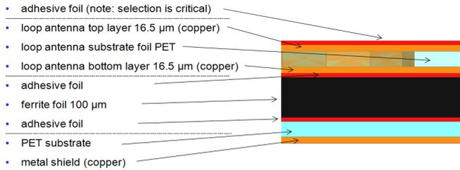
Fig. 7. Layer stack of prototype industrial NFC ALM antenna.
