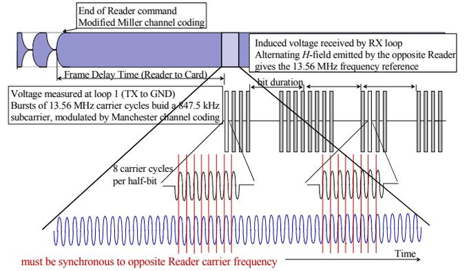
Fig. 8. Communication according ISO/IEC14443A BDR in ALM mode.
