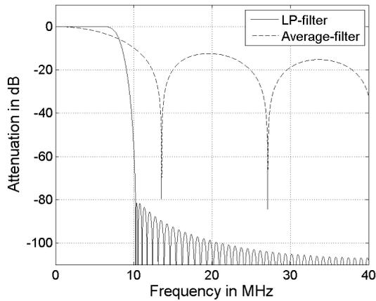
Figure 6. Low-pass-filters spectral transfer function.
