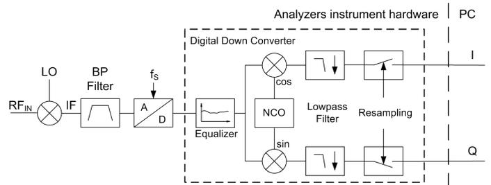
Figure 2. Signal processing chain of the signal analyzer, modified [9].
