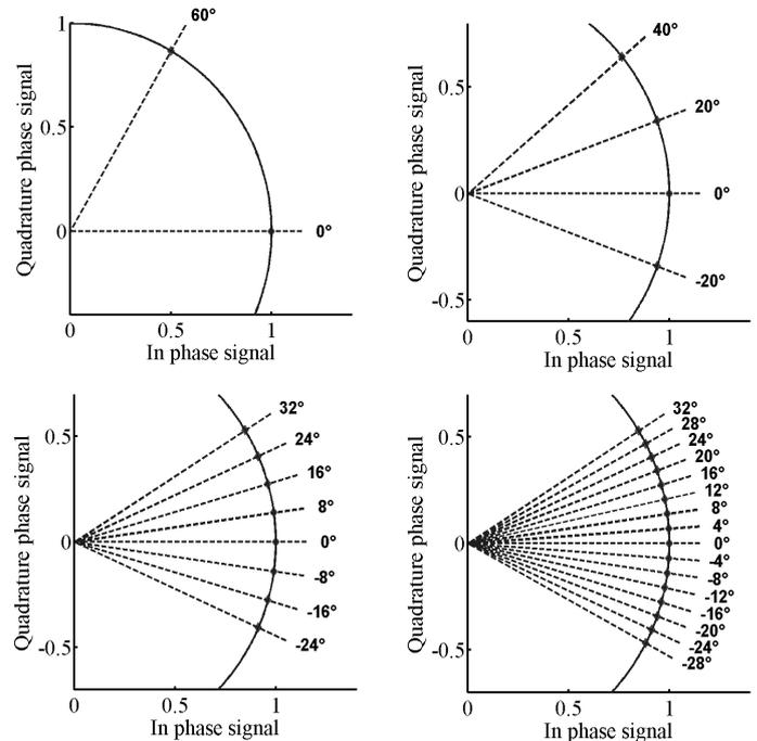
Figure 1. Constellation diagrams showing IQ segment and symbol positions of 2PSK, 4PSK, 8PSK and 16PSK (top left to bottom right), taken from [1].
