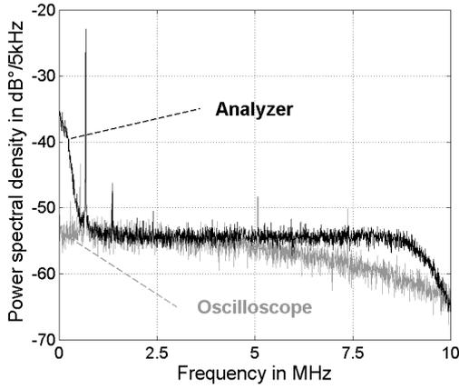
Figure 11. Phase noise spectrum comparison.
