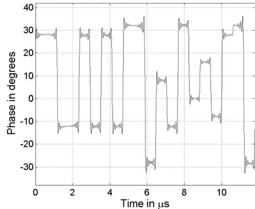
Figure 7. 16PSK8 communication sequence captured with analyzer.
