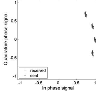
Figure 12. 4PSK2 constellation diagram measured with analyzer.
