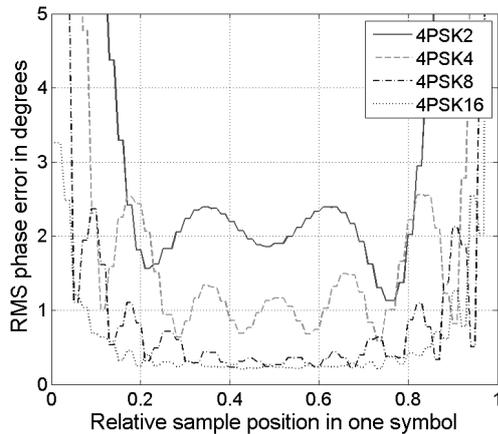
Figure 9. Phase error vs. sampling position for the analyzer.
