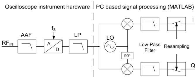
Figure 3. Signal processing chain of the digital sampling oscilloscope.
