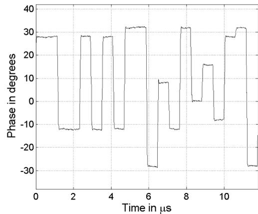
Figure 8. 16PSK8 communication sequence captured with scope.
