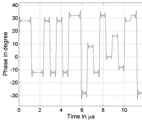
Figure 14. 16PSK8 time domain low-pass filtered, simulated.
