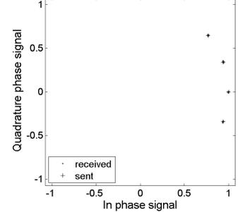
Figure 13. 4PSK2 constellation diagram measured with oscilloscope.
