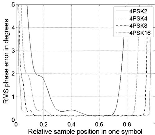
Figure 10. Phase error vs. sampling position for the oscilloscope.
