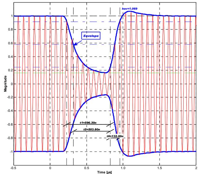
Figure 4 - ISO/IEC14443-2A interrogator modulation measurement and evaluation based on the proposed envelope detection and filtering method, data rate 424 kbit/s type A.
