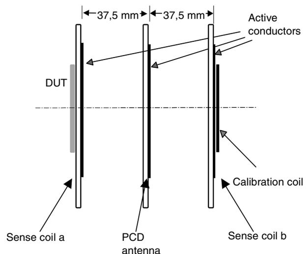
Figure 1 - Antenna arrangement for transponder test.
