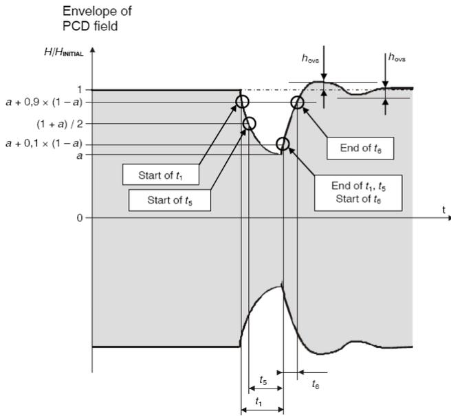
Figure 2 - ISO/IEC14443-2A HDR interrogator modulation evaluation and thresholds, taken from [10].
