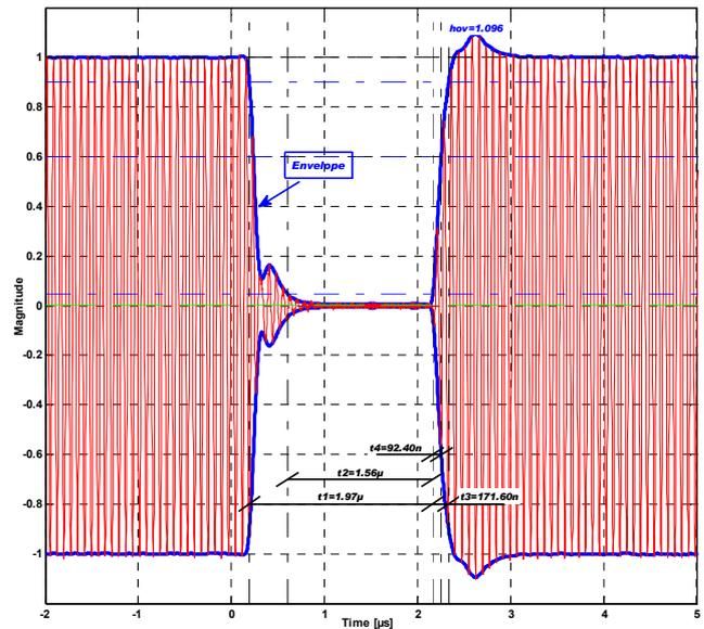
Figure 3 - ISO/IEC14443-2A interrogator modulation measurement and evaluation based on the proposed envelope detection and filtering method, data rate 106 kbit/s, type A.
