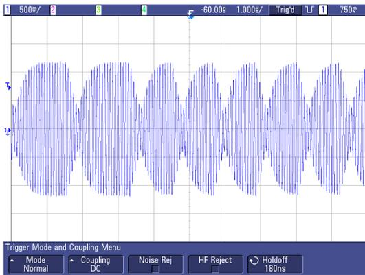
**Fig. 15:** Reader pulse shape properties of 14443-2 Type-A communication at 848 kbit/s (1 µs/Div.).
