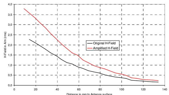
**Fig. 13:** Reader H-field vs. operating distance.
