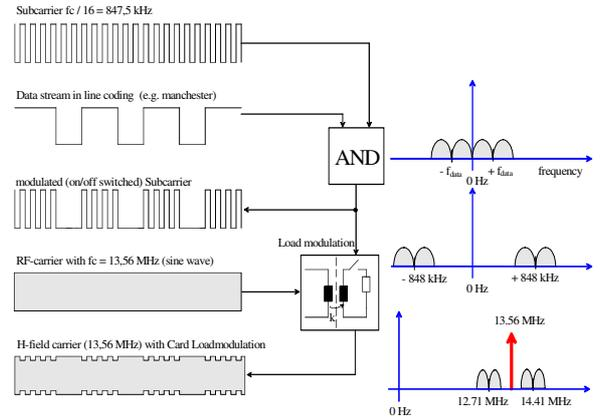
**Fig. 3:** Data transmission using load-modulation (ISO/IEC 14443, type A).
