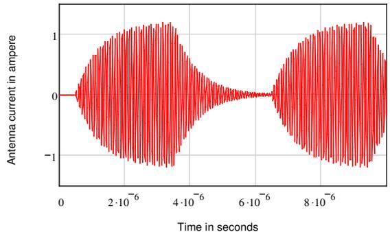
**Fig. 7:** Downlink data transmission pulses for reader antenna of  $Q = 60$ .
