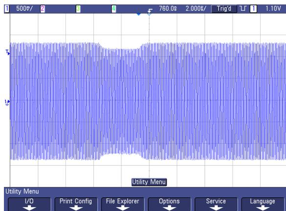
**Fig. 16:** Pulse shape properties of ISO/IEC 14443-2 Type-B communication (1 µs/Div.).
