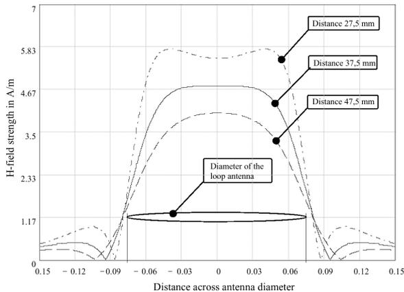
**Fig. 5:**  $H$ -field distribution over reader antenna.
