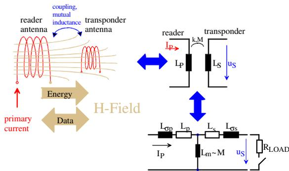
**Fig. 2:** Air interface principle of inductive coupled RFID Systems [6].
