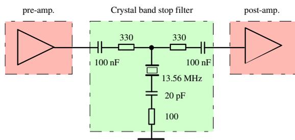
**Fig. 10:** Band stop filter (typical component values included).
