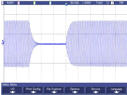
**Fig. 14:** Reader pulse shape properties of 14443-2 type A communication at 106 kbit/s (1 µs/Div.).
