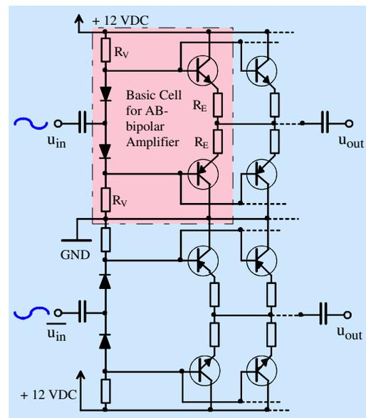
**Fig. 8:** 13.56 MHz AB Amplifier in a four-quadrant operation.
