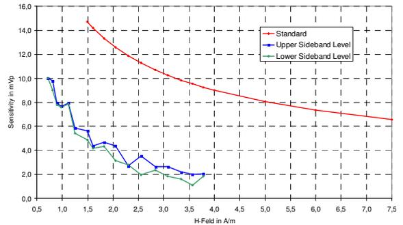
**Fig. 17:** Sensitivity vs. H-Field.
