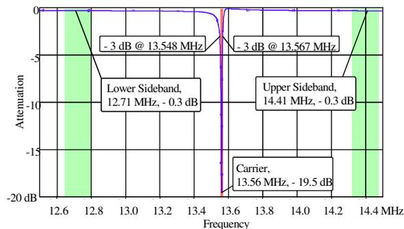
**Fig. 11:** Quartz band stop frequency response.
