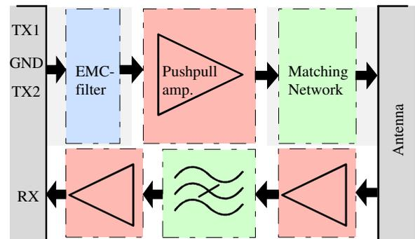
**Fig. 12:** Overall block diagram.
