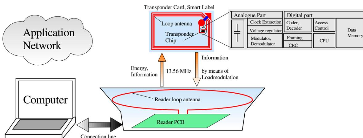
Fig. 1: Proximity RFID System concept.
