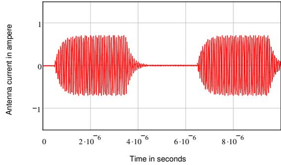
**Fig. 6:** Downlink data transmission pulses for reader antenna of  $Q = 20$ .
