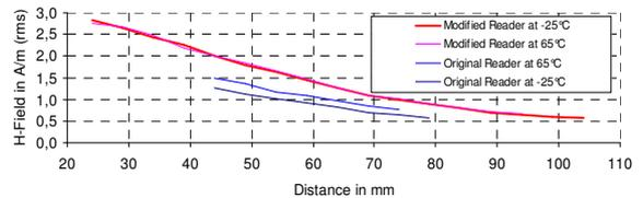
**Fig. 18:**  $H$ -Field vs. distance in mm at - 25°C and 65°C.
